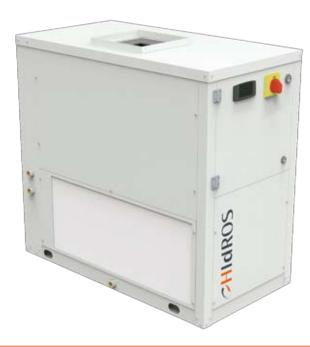
Series SDA dehumidifier are expressly designed for use in swimming pools where humidity should be closely controlled in order to guarantee optimal comfort. These units are intended to be installed in a technical room close to the swimming pool. A centrifugal fan with high available static pressure allows unit connection to ductworks, both for air suction and discharge. This series comprises 5 basic models which cover a capacity range from 73 to 250 I/24h.
